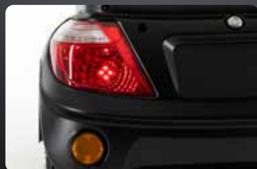
LED brake lights and turn signals
